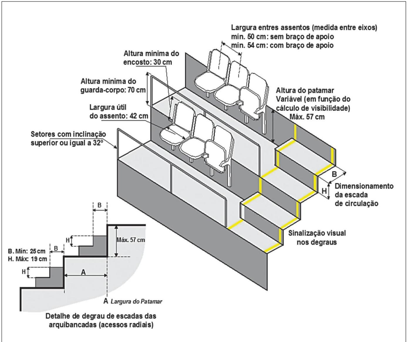
**FIGURA 4: DIMENSÕES DOS CORRIMÃOS E GUARDA-CORPOS DAS ESCADAS**
