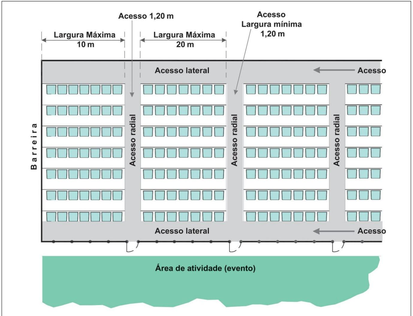
**FIGURA 2: BARREIRAS, GUARDA-CORPOS E CORRIMÃOS CENTRAIS: CARGAS DE PROJETO, ALTURAS E DISPOSIÇÕES**
